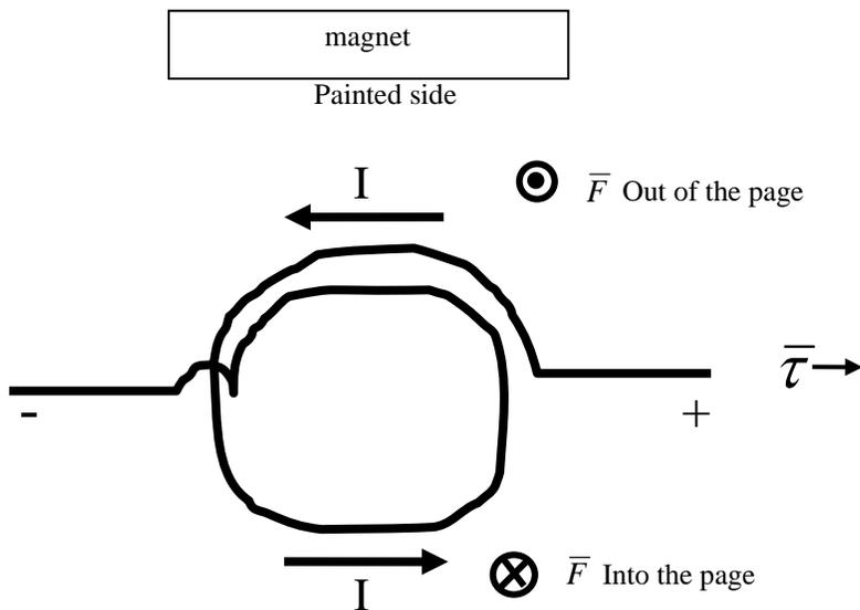
From this diagram you should be able to determine that the top of the coil is coming out of the page, and the bottom of the coil is going into the page. Applying  $\vec{F} = I\vec{L} \times \vec{B}$  at the very top and very bottom of the coil, it can be determined that the magnetic field,  $\vec{B}$ , supplied by the magnet is pointing down; therefore, the painted side of the magnet is the North Pole of the magnet.
