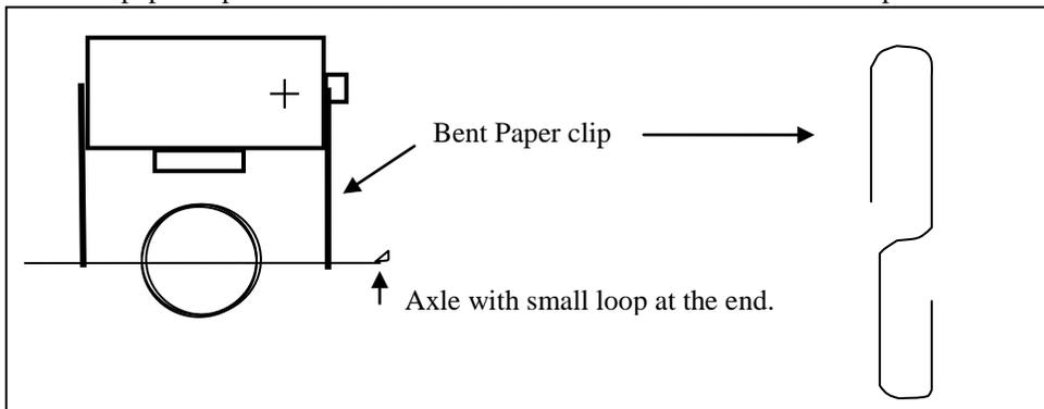
8. While holding the paper clips in place with your thumb and finger, slide the coil into position under the battery/magnet. Do not tape or otherwise force the paperclips to stay on the batteries. Hold the paperclips in place with your finger and thumb. **If your battery is returned damaged either by peeling the label or in any way exposing the end of the terminals, your grade will be reduced by 25 points. If you do not turn in your magnet, you will also lose 25 points.**
